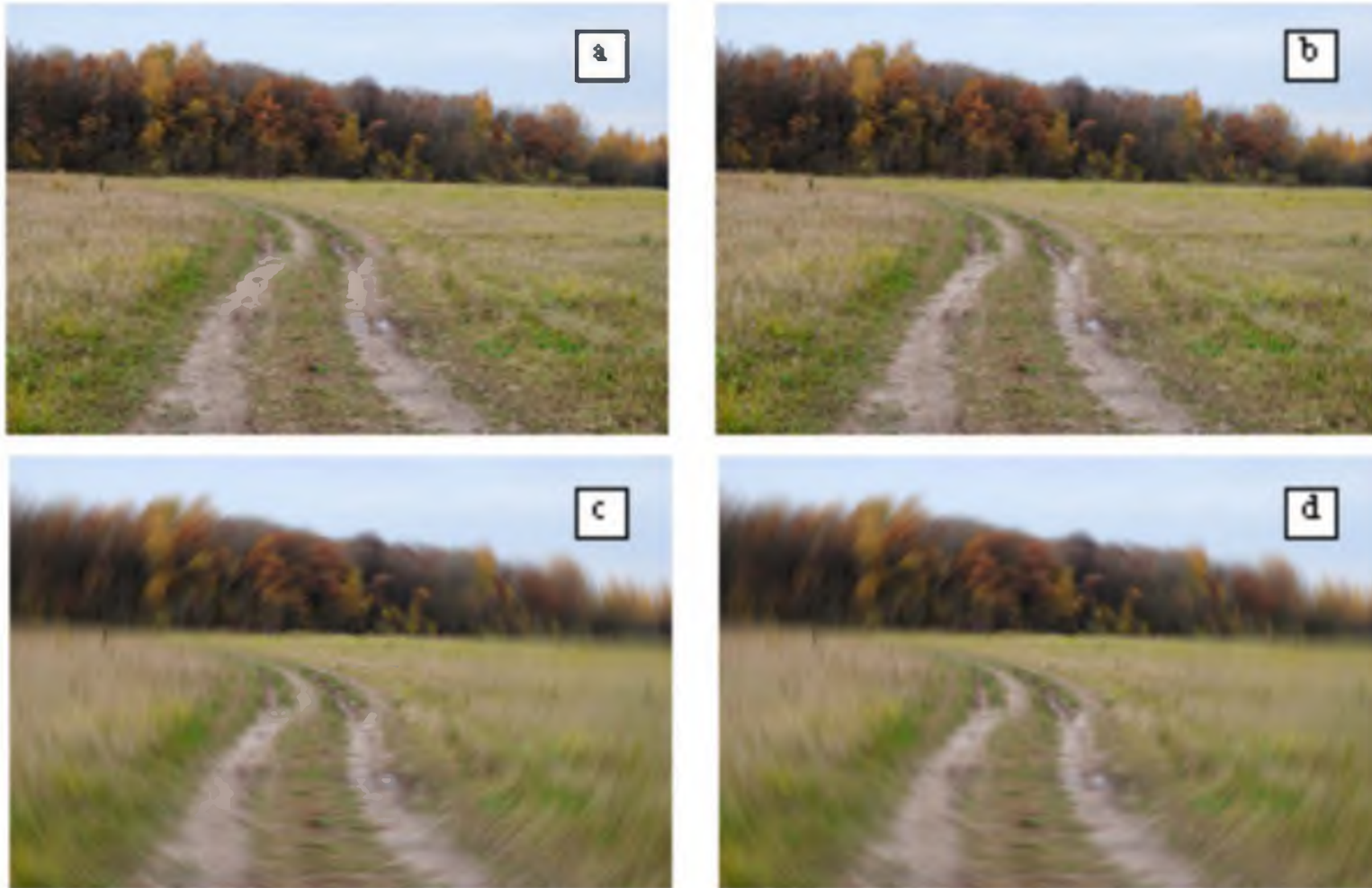
Fig. 4 a shows initial image, obtained from unmoving MR; fig. 4 b shows image, when trunk has longitudinal oscillations, fig. 4 c shows image, when trunk has transverse oscillation, and fig. 4 c combine longitudinal and transverse oscillations of trunk.
