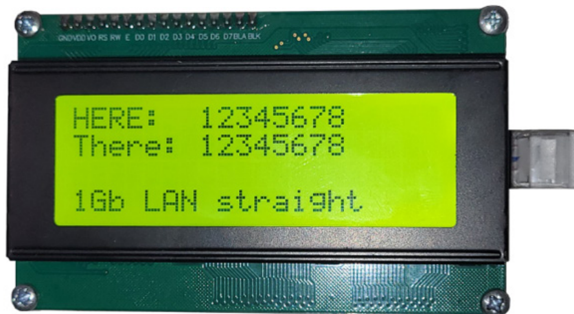
Fig. 2. The result of the device operation. Direct crimp cable connected
