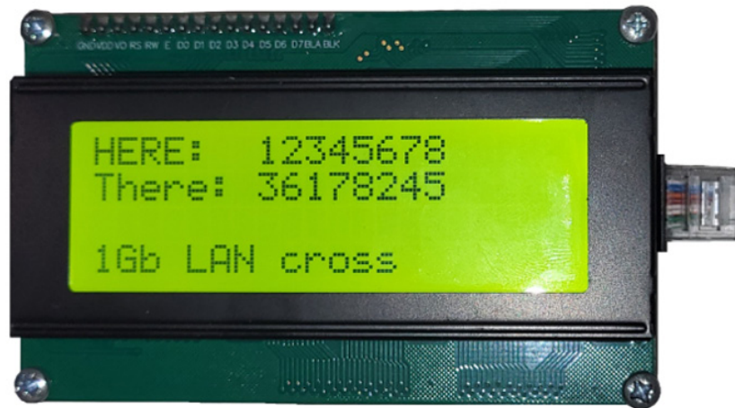
Fig. 3. The result of the device layout. Cross-crimped cable connected
