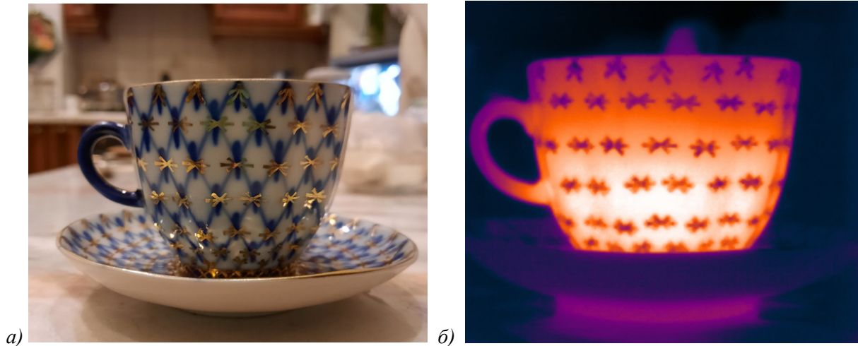
Fig. 5 – Image of a porcelain cup with a pattern: a) – in the visible spectrum, b) – in the infrared spectrum
