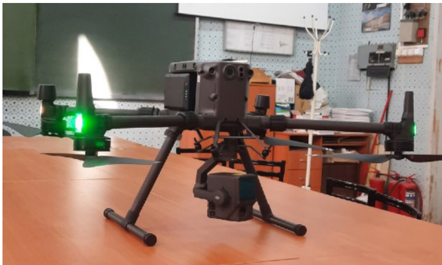
Fig. 1. UAV with lidar installed on it
