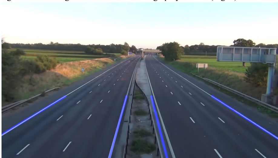
Fig. 5 – The result of the search for highway markings
