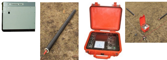
Fig. 2: "Kola" generating and measuring complex ULF, ELF, VLF range for radio physical and geophysical exploration [1]
