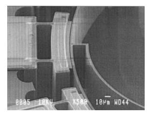
Fig. 4. SEM view of the capacitive gap between the electrode and the ring
