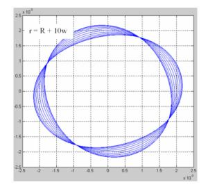
Fig. 7. Evolution of the elliptic vibrations form
