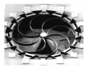
Fig. 2. SEM view of micromechanical vibrating ring gyroscope
