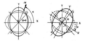
Fig. 3. Vibrations of a wave micromechanical gyroscope when there is no rotation of sensor (left) and when sensor is rotating (right)
