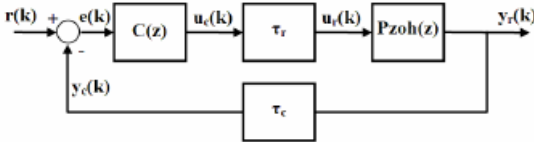
Fig. 4a. Block Diagram with delays in both control and feedback line
